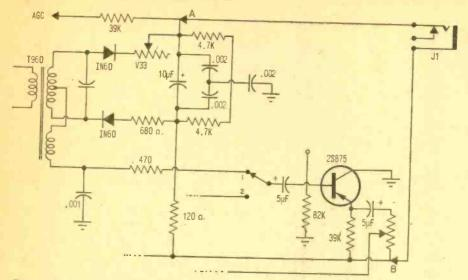
Fig. 1. Ratio detector circuit of Radio Shack Patrolman. The only modification of receiver to accommodate squelch is addition of jack J1 wired to points A and B.
