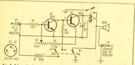
Fig. 2. Schematic diagram of Shush Box. Circuit functions as a simple amplifier energizing relay K1 whenever receiver picks up a signal.
