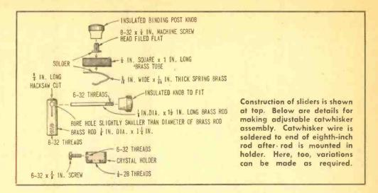
catwhisker, but steel, phosphor bronze, and tungsten wires were also used in the old days. The business end of the catwhisker wire should be pointed with a file. For the detector, you can use a mounted galena or silicon crystal.
