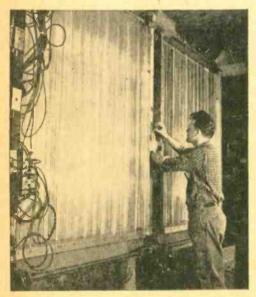
Charged atomic particles passing through this spark chamber cause high voltage sparks to jump from plate to plate, thus revealing the path of the speeding particles.
