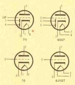
the 6-prong socket with an octal type. If memory serves me right, a 76 is a triode which can be replaced with a 6J5GT. Replace the 5-prong socket with an octal type. The diagram shows the difference in socket connections.
