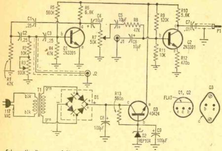
Schematic diagram of Throb Maker, an easy-to-build add-on tremolo adapter.
