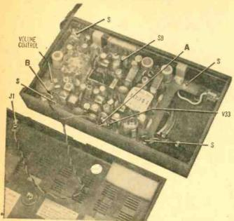
aluminum chassis box. Fortunately, parts are not very crowded and assembly and wiring aren't difficult. In short, the layout isn't critical and almost any arrangement of parts that proves convenient can be used.
