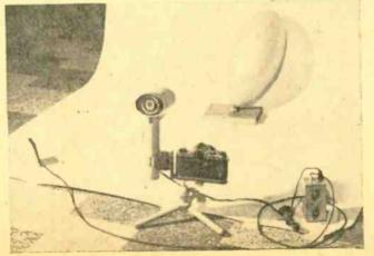
Second Splitter hooked up to camera and electronic flash ready to catch the action of the balloon being punctured.
