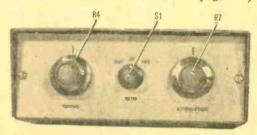
Finished Hum Bug, willing and able to go to work knocking the audibility out of hum. Front-panel controls provide for tuning frequency and adjusting level of rejection notch.
