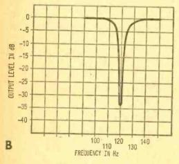
63 Hz are less than 3 dB down). In effect, the hum is removed with no noticeable effect on the remaining low-frequency sound. When 120-Hz hum is being filtered, the 3-dB-down points are 115 and 125 Hz; again, little sound is lost other than at the hum frequency.
