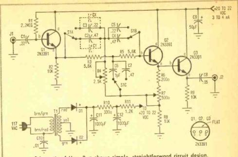
Schematic of Hum Bug shows simple, straightforward circuit design.
