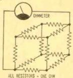
Here's the resistive cube! Now figure out the ohmmeter reading!
