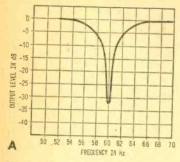
Hum Bug's sharp rejection of 60- and 120-Hz hum frequencies is shown in curves A and B, respectively. Positive feedback increases effective Q sharpness of parallel-T filter.
